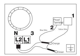
Do not wire the valve switch to close a circuit that will directly power another safety shutoff valve. Doing so could result in a safety valve being energized and opened rather than remaining closed.
